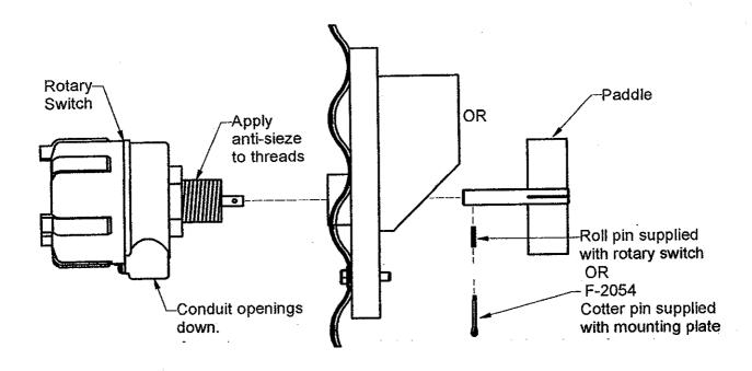
7) Install the paddle using either the roll pin or cotter pin supplied. If using the roll pin, start it into the paddle first, then when it is on the rotary switch shaft, use pliers to push it all the way through. Don't use a hammer, as this may damage the bearings in the rotary switch.
