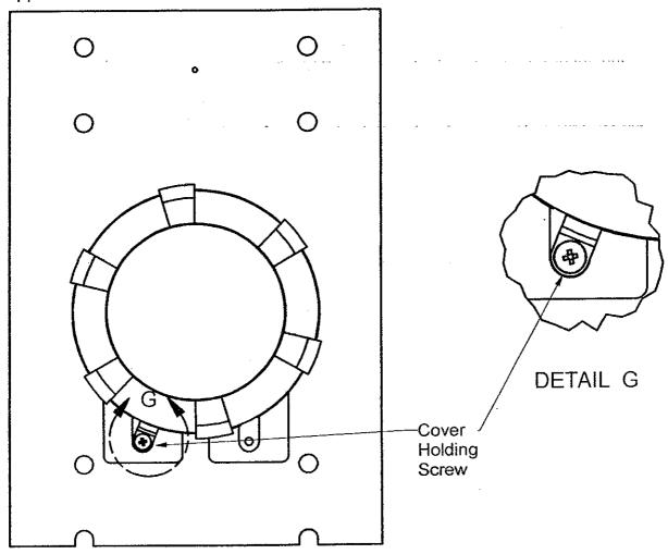
9) When wiring is complete, apply anti-sieze to cover threads and screw cover onto switch. Lock cover in place by tightening cover holding screw.
