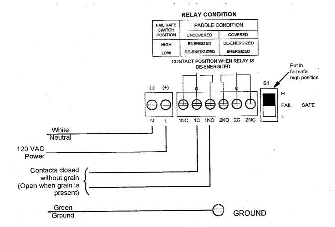
For replacement of Shivvers Low Grain Shut-Off (LGSO) or Grain Level Indicator (GLI).
