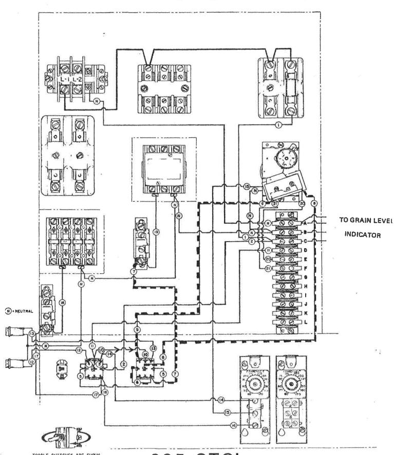
TOGGLE SWITCHES ARE SHOWN IN CORRECT POSITION BUT ROTATED 180° RIGHT TO LEFT. THIS REVERSES THE SIDE THE TERMINALS ARE ON.
